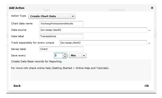
In this example, we are tracking transaction failures per client over time. We call the chart data "ExchangeTransactionResults" and we are tracking a separate data series for each individual client.
